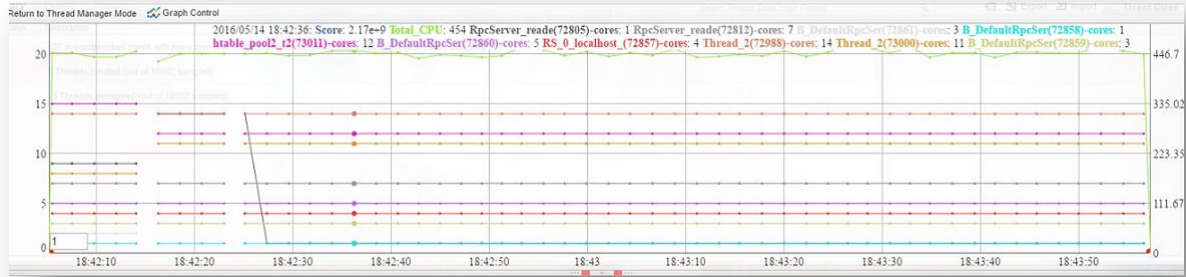
Figure 7 Thread Positions over time for T-004 (6596.506 ops/sec - T-001 gain baseline gain = 65.44%
